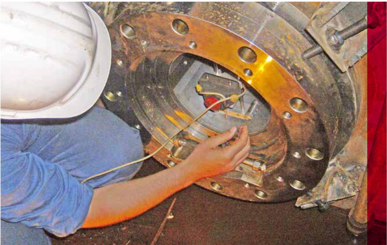
**Laser alignment of sterntube bearings.**
