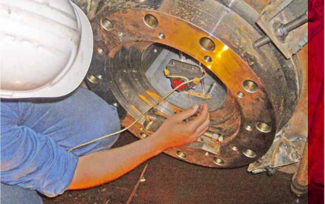
Laser alignment of sterntube bearings.
